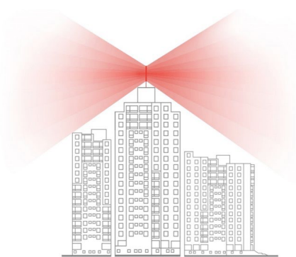
Figure 3.1 – Correct antenna installation position
